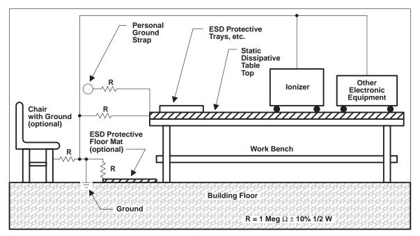
All electrical equipment sitting on the conductive table top must be hard grounded but must be isolated from the static dissipative work surface.
