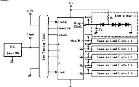
Notes) 1.  $C_L$  includes probe and jig capacitance. 2. All diodes are 1S2074 H.
