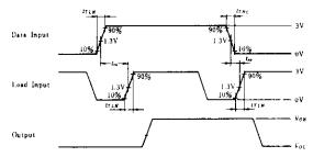
Input pulse:  $t_{TLH}$ ,  $t_{THL} \le 10$ ns, PRR = 1MHz, Duty cycle  $\le 50\%$
