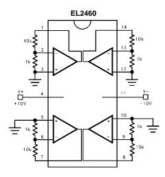
Differential Gain and Phase Test Circuit
