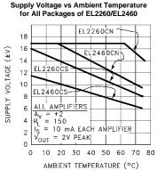
The curves do not include heat removal or forcing air, or the simple fact that the package will probably be attached to a circuit board, which can also provide some form of heat removal. Larger temperature and voltage ranges are possible with heat removal and forcing air past the part.
