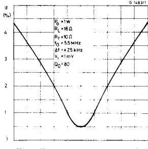
Fig. 3 – Amplitude modulation rejection vs. input signal power
