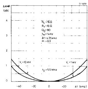
Fig. 7 – Distortion vs. frequency deviation
