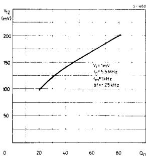
Fig. 8 – Distortion vs. tuning frequency change
