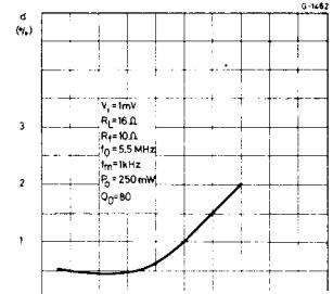
Fig. 2 – Output voltage attenuation vs. DC volume control resistance
