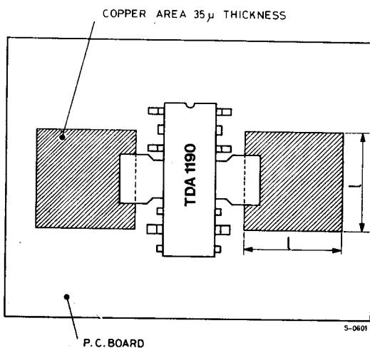
Fig. 19 – External heatsink mounting example
