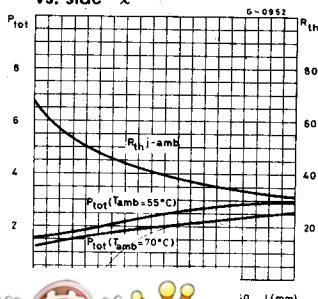
Fig. 21 – Maximum allowable power dissipation vs. ambient temperature
