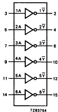
Fig.4 Functional diagram.
