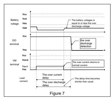
Even if the state change to overdischarge condition, the battery package capacity is same as typical.
