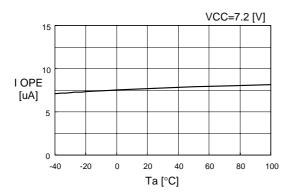
Current consumption vs. temperature in power-down mode
