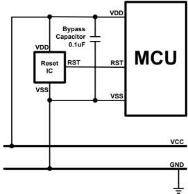
The external reset circuit also use external reset IC to enhance MCU reset performance. This is a high cost and good effect solution. By different application and system requirement to select suitable reset IC. The reset circuit can improve all power variation.
