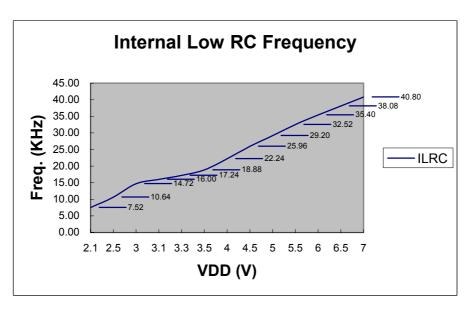
The internal low RC supports watchdog clock source and system slow mode controlled by CLKMD.
