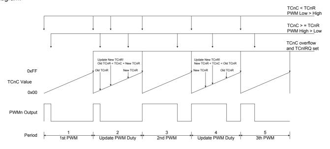
In period 2 and period 4, new Duty (TCnR) is set. TCn is double buffer design. The PWM still keeps the same duty in period 2 and period 4, and the new duty is changed in next period. By the way, system can avoid the PWM not changing or H/L changing twice in the same cycle and will prevent the unexpected or error operation.
