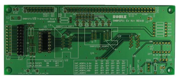
U2: Set SOP 14 pin socket for SN8P2711S programming (using SOP 16 pin socket: TX-SOP16PIN).
