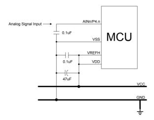
ADC reference high voltage is from VDD pin and AIN0/P4.0 is VERFH input. The VERFH should be from MCU's VDD pin. Don't connect from main power.
