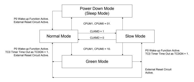
**System Mode Switching Diagram**
