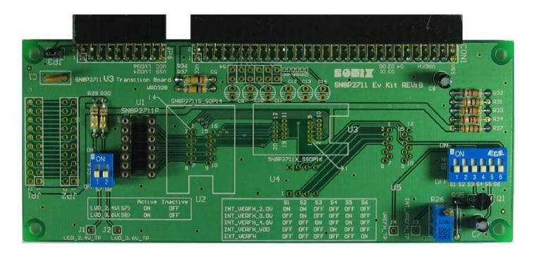
CON1: I/O port and ADC reference input. Connect to SN8ICE 2K CON1.
