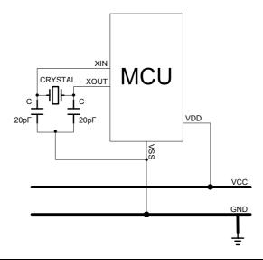
Note: Connect the Crystal/Ceramic and C as near as possible to the XIN/XOUT/VSS pins of micro-controller.
