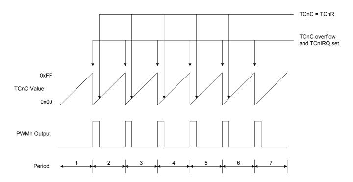
Above diagram is shown the waveform with fixed TCnR. In every TCnC overflow PWM output "High, when TCnC≧ TCnR PWM output "Low". If TCnR is changing in the program processing, the PWM waveform will became as following diagram.
