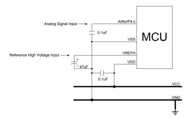
ADC reference high voltage is from external voltage and AIN0/P4.0 is VERFH input. The capacitor (47uF) between VREFH and VSS is necessary to stable VERFH voltage.
