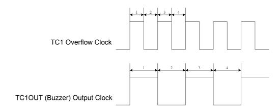
Example: Setup TC10UT output from TC1 to TC10UT (P5.3). The external high-speed clock is 4MHz. The TC10UT frequency is 0.5KHz. Because the TC10UT signal is divided by 2, set the TC1 clock to 1KHz. The TC1 clock source is from external oscillator clock. TC1 rate is Fcpu/4. The TC1RATE2~TC1RATE1 = 110. TC1C = TC1R = 131.
