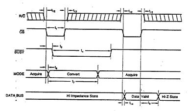
Using CS and BYTE to Control Data Bus.
