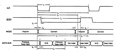
Using CS to Control Conversion and Read Timing.
