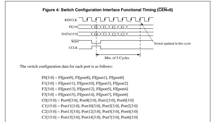
Where FI[portN] is the Force IDLE bit for port N and PortN[3:0] is the input port number to be connected to output port N.
