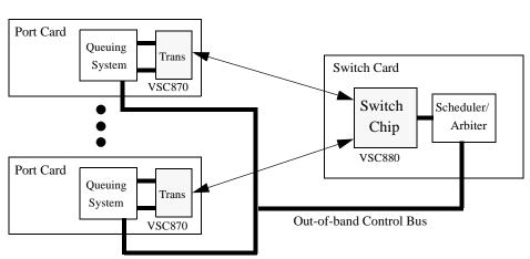
Figure 8: Cell Based System
