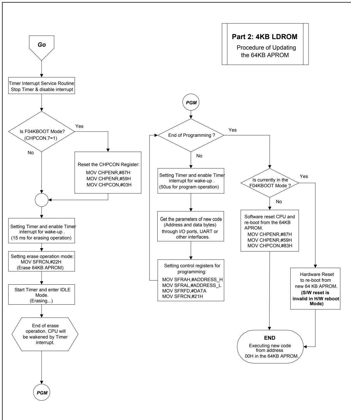
Figure 15-2 The algorithm of ISP for LD ROM
