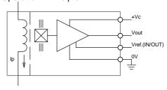
(\*) should be connected to 0V of Power Supply for better dv/dt immunity. Arrow indicates positive current direction.
