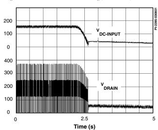
Figure 13. Slow Power-Down Timing with Optional External (4  $M\Omega$ ) UV Resistor Connected to EN/UV Pin. WWW.DataSheet4U.com
