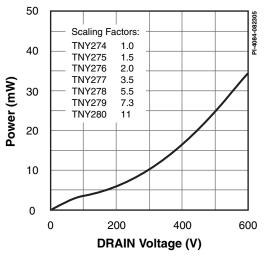
Figure 26. Drain Capacitance Power.
