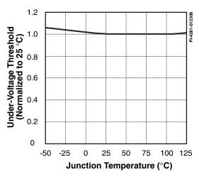
Figure 27. Under-Voltage Threshold vs. Temperature.
