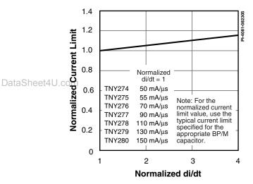
Figure 23. Current Limit vs. di/dt.
