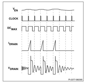
Figure 8. Operation at Medium Loading.
