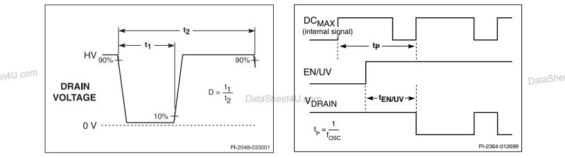
Figure 17. Duty Cycle Measurement.
