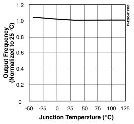
Figure 21. Frequency vs. Temperature.
