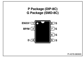
Figure 3. Pin Configuration.
