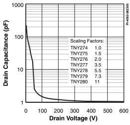
Figure 25.  $C_{oss}$  vs. Drain Voltage.
