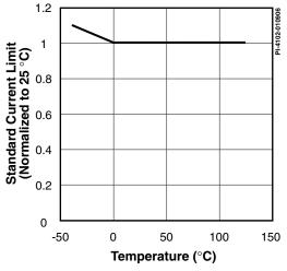
Figure 22. Standard Current Limit vs. Temperature.
