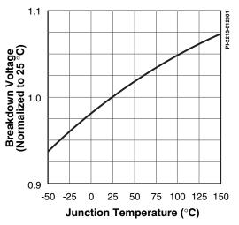
Figure 20. Breakdown vs. Temperature.
