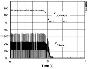
Figure 12. Normal Power-Down Timing (without UV).
