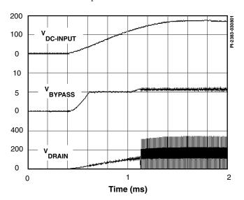
Figure 10. Power-Up with Optional External UV Resistor (4  $M\Omega$ )
