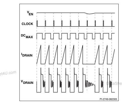
Figure 6. Operation at Near Maximum Loading.
