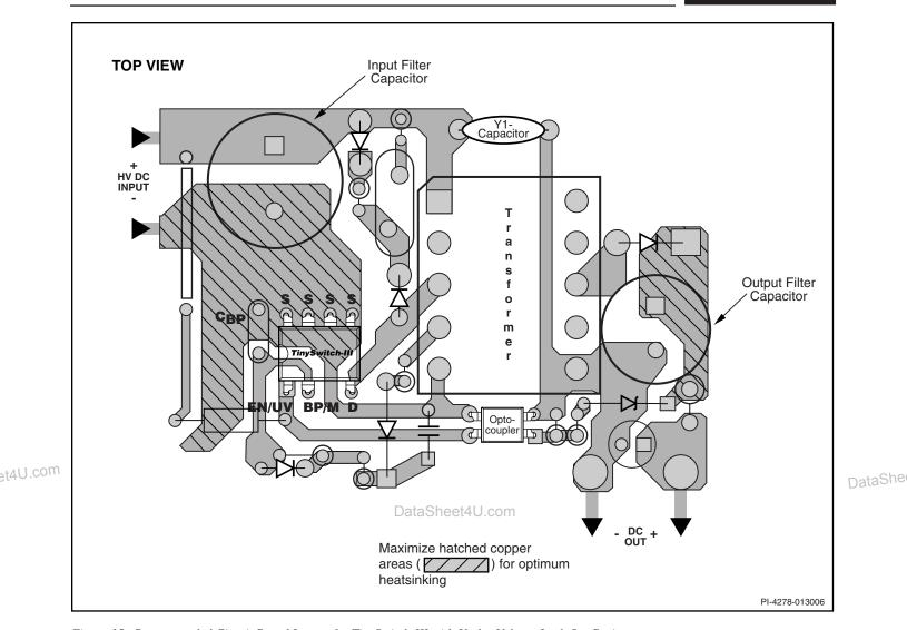
Figure 15. Recommended Circuit Board Layout for TinySwitch-III with Under-Voltage Lock Out Resistor.
