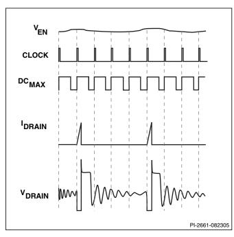
Figure 9. Operation at Very Light Load.
