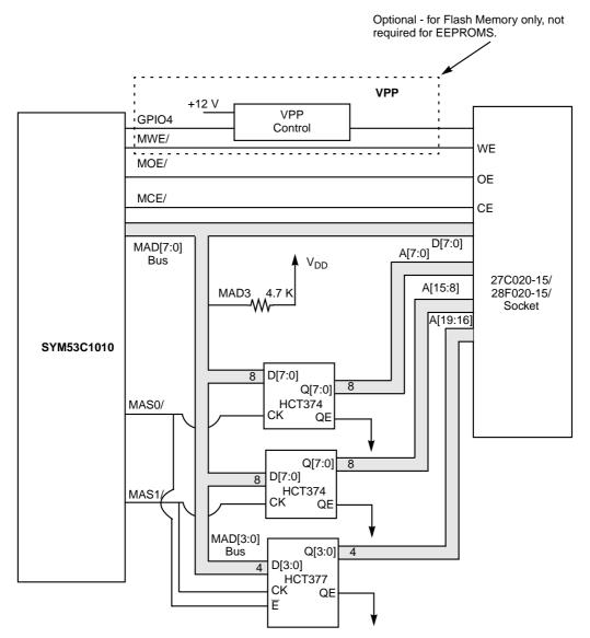
Note: MAD[2:0] pulled low internally. MAD bus sense logic enabled for 128, 256, 512 Kbytes, or 1 Mbyte of fast memory (150 ns devices @ 33 MHz). The HCT374s may be replaced with HCT377s.
