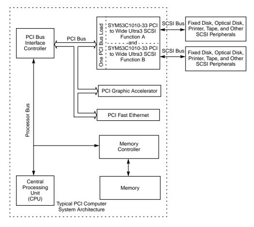
Figure 1.2 Typical SYM53C1010-33 System Application
