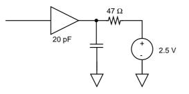
Figure 6.4 SCSI Input Filtering
