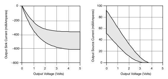
Figure 6.7 Output Current as a Function of Output Voltage
