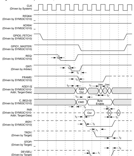
Figure 6.18 Burst Opcode Fetch, 32-Bit Address and Data
