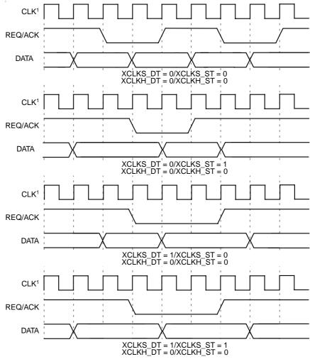
Figure 4.2 Double Transition Transfer Waveforms (XCLKS Examples)
