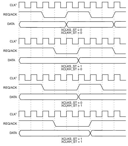
Figure 4.1 Single Transition Transfer Waveforms
