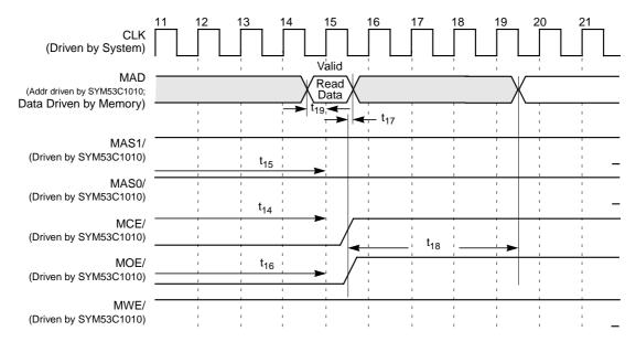
Figure 6.27 Normal/Fast Memory (≥ 128 Kbytes) Single Byte Access Read Cycle (Cont.)
