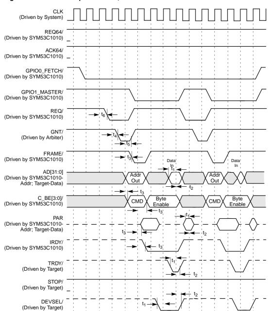
Figure 6.17 Nonburst Opcode Fetch, 32-Bit Address and Data
