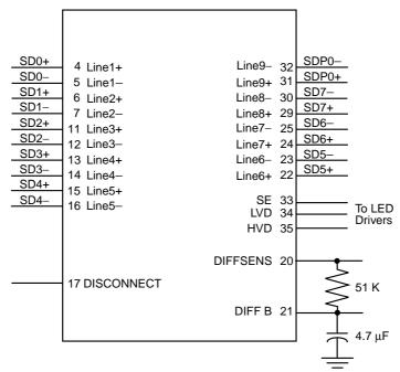
Figure 2.4 Regulated Termination for Ultra3 SCSI
