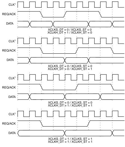
Figure 4.3 Double Transition Transfer Waveforms (XCLKH Examples)
