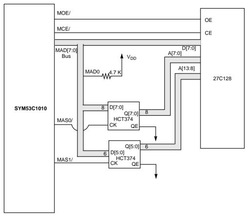
Note: MAD[3:1] pulled low internally. MAD bus sense logic enabled for 16 Kbyte of slow memory (200 ns devices @ 33 MHz).
