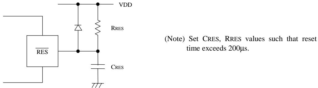
Figure 5 Reset circuit
