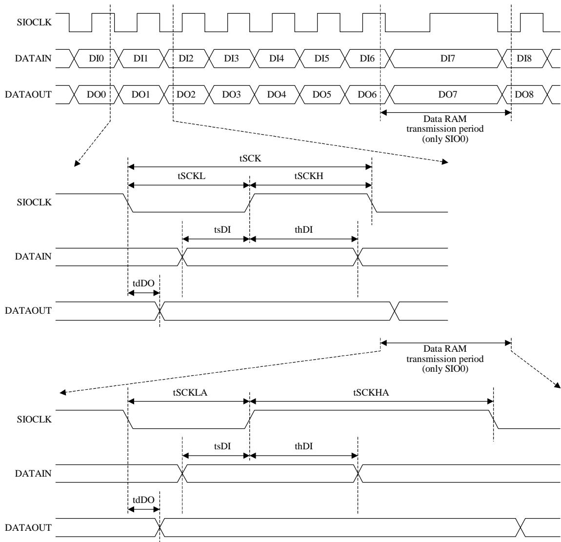
Figure 6 Serial input / output test condition
