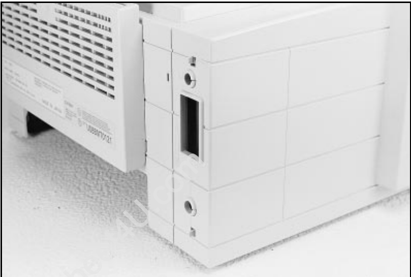
Figure 15 5P/5MP I/O Cover Release Tabs
