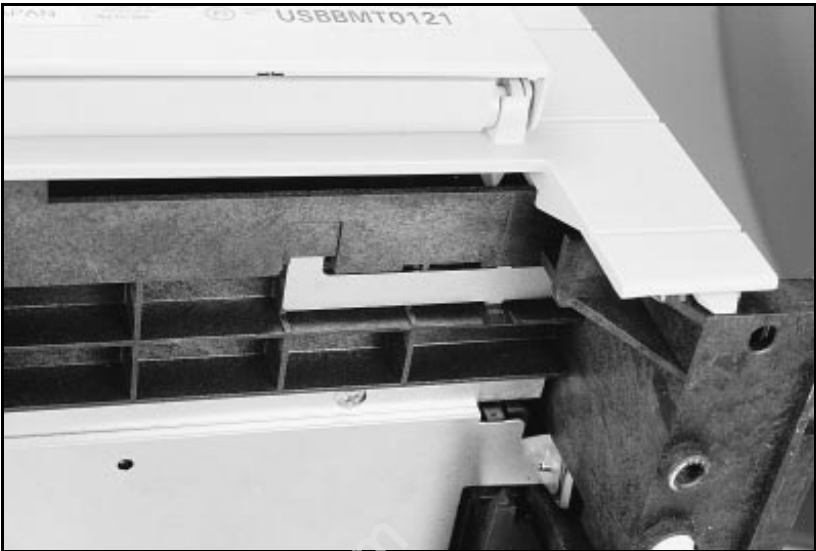
Figure 19 Releasing the Back Corner of the Top Cover
