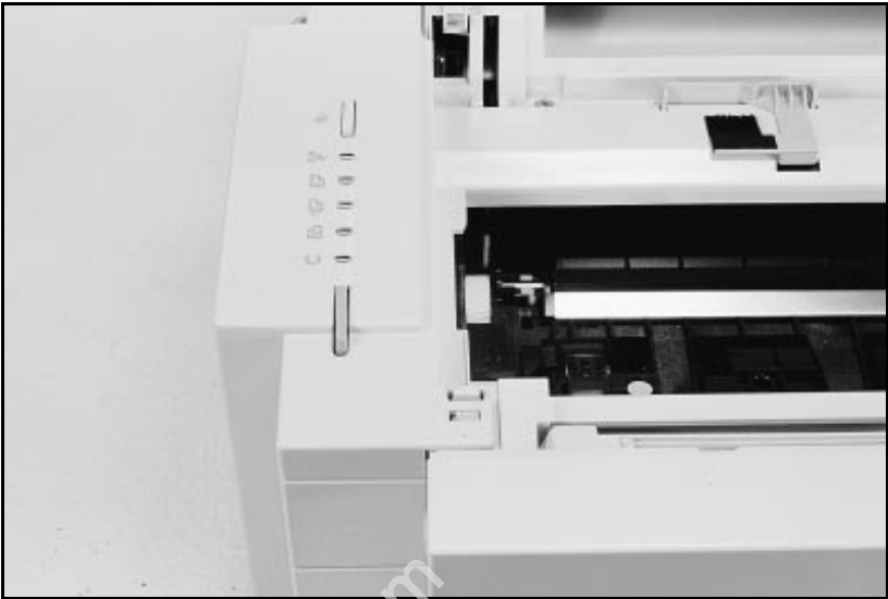
Figure 17 Left Side Cover Release Latch (5P/5MP shown)
