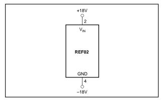
FIGURE 1. Burn-In Circuit.
