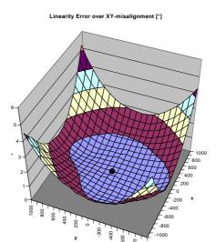
Figure 20: Example of linearity error over XY misalignment
