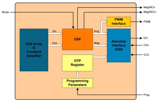
Figure 3: AS5045 block diagram
