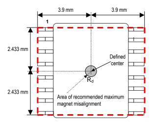
Figure 17: Defined chip center and magnet displacement radius
