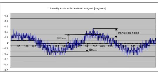
Figure 21: Example of linearity error over 360°
