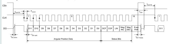
Figure 4: Synchronous serial interface with absolute angular position data
