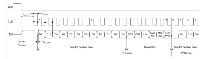
Figure 6: Daisy Chain mode data transfer
