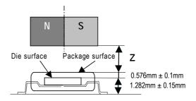
Figure 18: Vertical placement of the magnet
