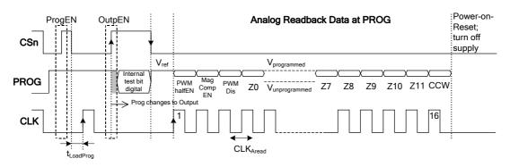
Figure 12: OTP register analog read
