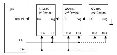
Figure 5: Daisy Chain hardware configuration
