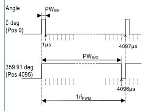
Figure 7: PWM output signal
