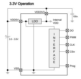
Figure 15: Connections for 5V / 3.3V supply voltages
