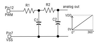
Figure 8: Simple 2nd order passive RC lowpass filter
