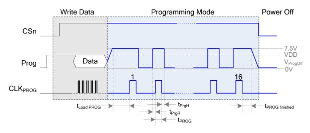
Figure 10: Complete programming sequence
