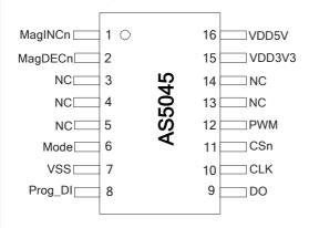
Figure 2: Pin configuration SSOP16
