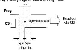
Figure 13: Enabling the alignment mode
