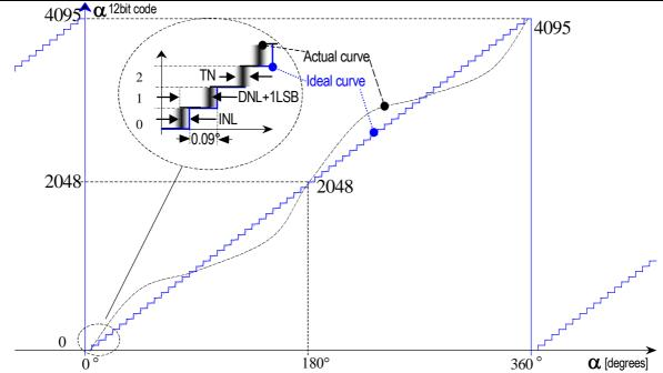
Figure 22: Integral and differential non-linearity (example)
