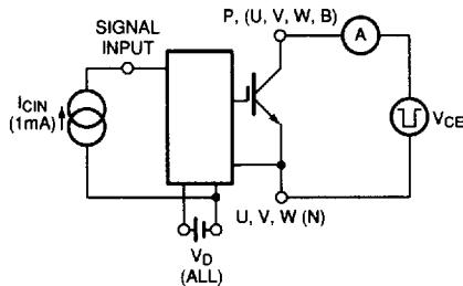
**Figure 6**  $I_{CES}$  Test
