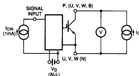
Figure 2  $V_{CE(SAT)}$  Test
