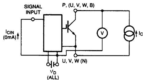
Figure 1  $V_{CES}$  Test
