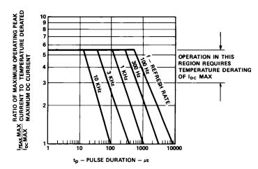
Figure 1. Maximum Allowable Peak Current vs. Pulse Duration.
