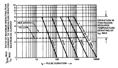
Figure 6. Maximum Allowed Peak Current vs. Pulse Duration.
