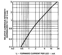
Figure 5. Relative Luminous Intensity vs. DC Forward
