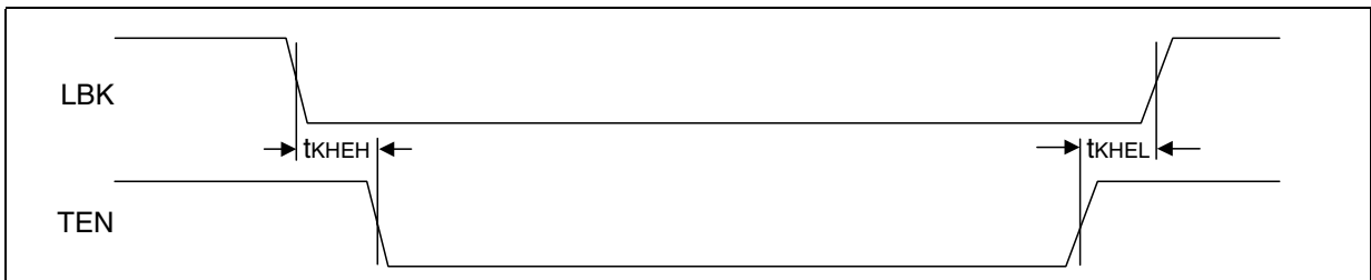
Figure 28. Mode 2 Loopback Timing
