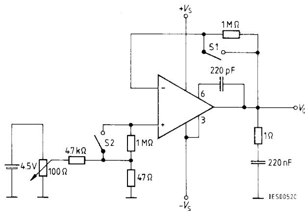
$$\text{S1 open - S2 closed: } I_{I-} = \frac{V_O}{1 \text{ M}\Omega}$$
