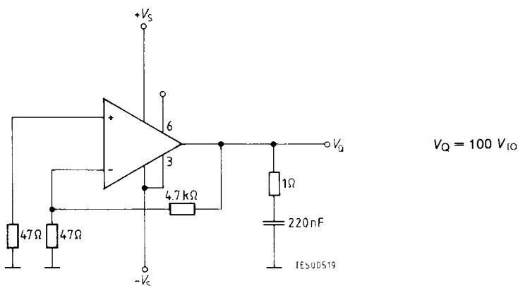
**Figure 3****Input Offset Current; Input Current, Temperature Coefficient of  $I_{IO}$**
