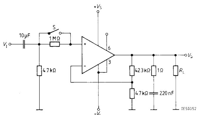
S closed: to measure  $V_{IO}$
