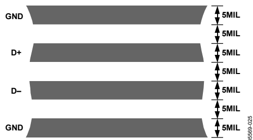
Figure 35. Typical Arrangement of Signal Tracks
