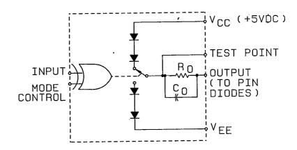
By utilizing an external current limiting structure (accessed via the test point terminal) asymmetrical output currents can be produced from symmetrical power supplies or symmetrical output currents from asymmetrical supplies.
