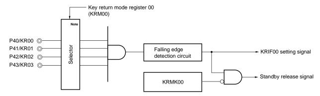
**Note** For selecting the pin to be used as falling edge input.
