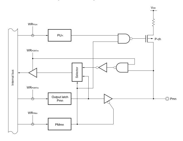
Caution Figure 5-2 shows the basic configuration of a CMOS I/O port. This configuration differs depending on the functions of alternate function pins. Also, an on-chip pull-up resistor can be connected to port 4 by means of a setting in key return mode register 00 (KRM00).
