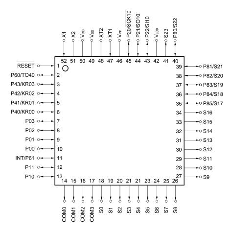
Caution In normal operation mode, directly connect the VPP pin to Vss.
