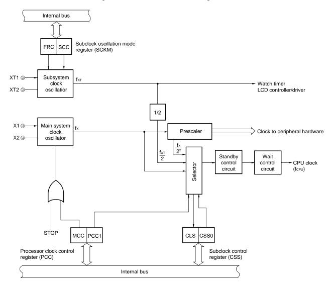
Figure 5-7. Clock Generator Block Diagram
