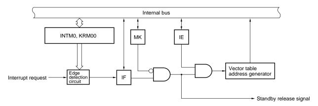
INTM0: External interrupt mode register 0 KRM00: Key return mode register 00
