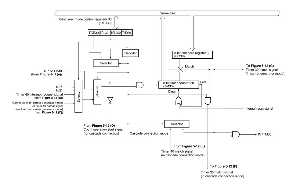
Figure 5-12. Block Diagram of Timer 40
