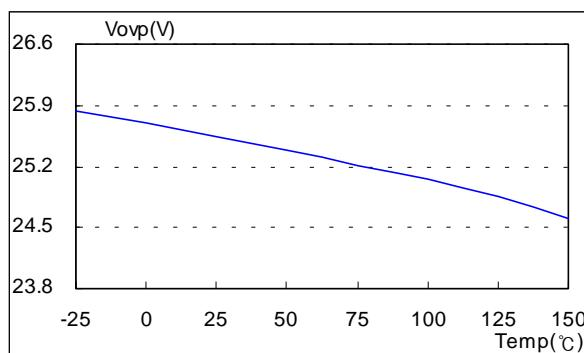
Figure 10. Over Voltage Protection vs. Temp.
