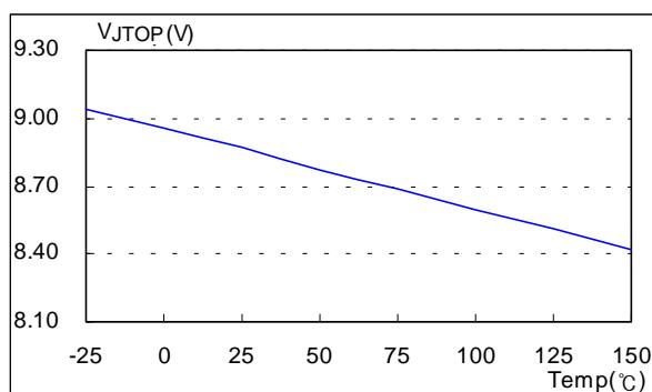
Figure 3. Stop Threshold Voltage
