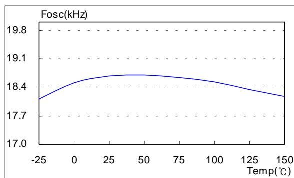
Figure 5. Initial Frequency VS. Temp
