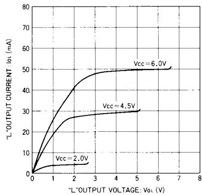
Fig. 8 Output low current vs. output low voltage
