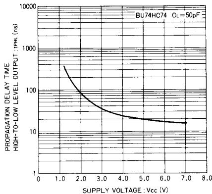
Fig. 14 High-to-low propagation delay time
