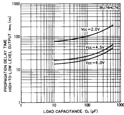
Fig. 18 High-to-low propagation delay time
