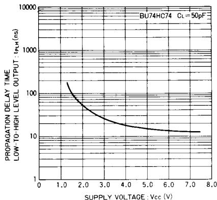
Fig. 13 Low-to-high propagation delay time
