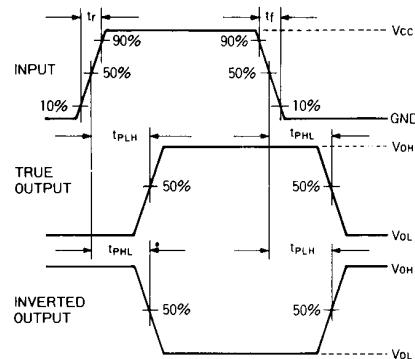
Fig. 48 Propagation delay time
