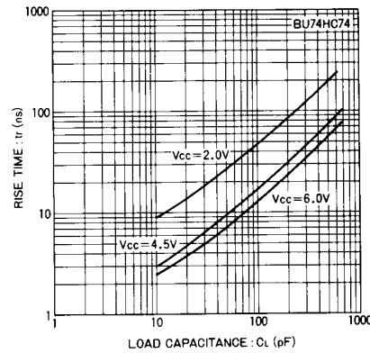
Fig. 15 Rise time vs. load capacitance
