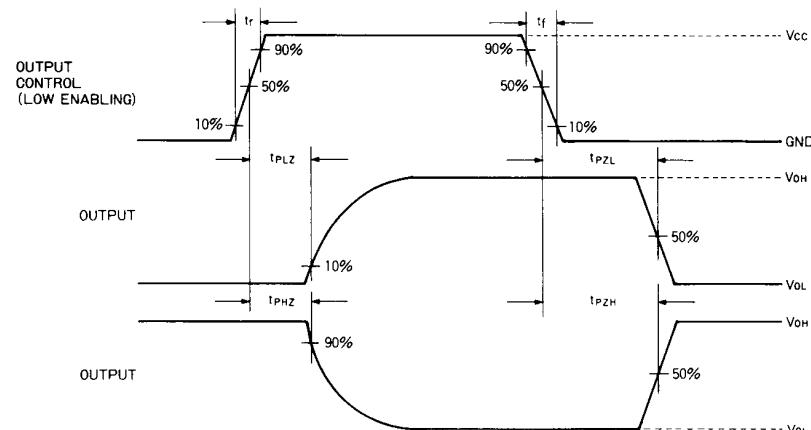
Fig. 51 Tristate output enable waveform,
