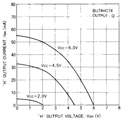
Fig. 7 Output high current vs. output high voltage
