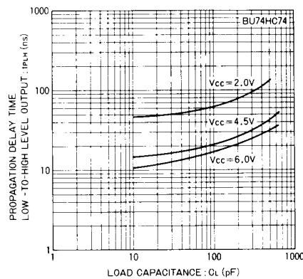
Fig. 17 Low-to-high propagation delay time
