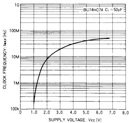
Fig. 10 Maximum clock frequency vs. supply voltage
