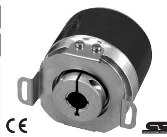
Pepperl+Fuchs' ASS58/ASM58 series absolute encoders feature recessed hollow shafts and communicate via SSI (synchronous serial interface). The encoder is mounted directly to the shaft using set screws. The torque rest is used to prevent the encoder from rotating. Available in either single-turn with 16-bit resolution, or multi-turn with 28-bit resolution versions. These encoders are rated IP65 and feature a rugged aluminum housing.
