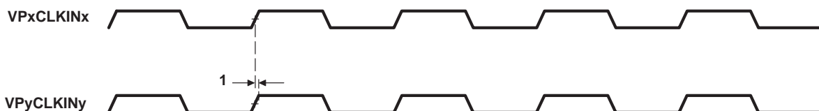
Figure 18–6. Video Port Dual-Display Sync Timing
