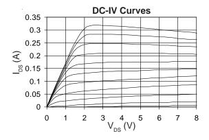
$V_{GS}$  = -2.0 to 0V, 0.2V steps T=25°C
