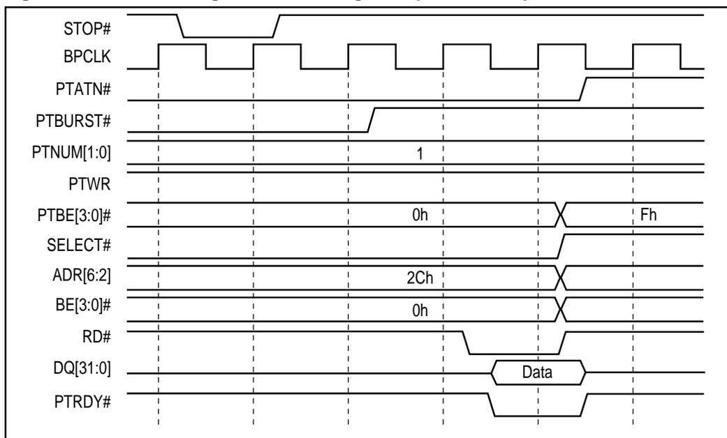
Internal byte lane steering may be used whether the MODE input defines a 16-bit or 32-bit Add-On interface. When a 16-bit Add-On interface is used, the ADR1 input is used in conjunction with the byte enables to steer data into the proper APTD register byte locations.
