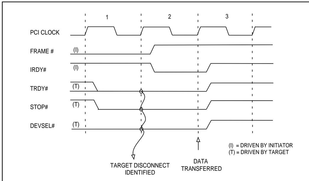
**Figure 10b. Target Disconnect Example 2 (IRDY# asserted)**
