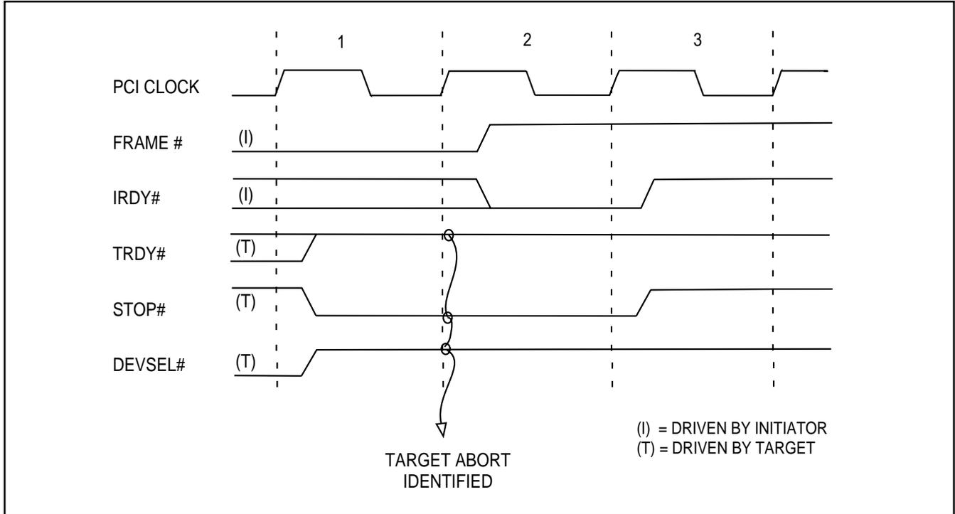
Figure 13. PCI Bus Arbitration and S5935 Bus Ownership Example
