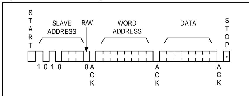
**Figure 4. Serial Interface Byte Access — Read**
