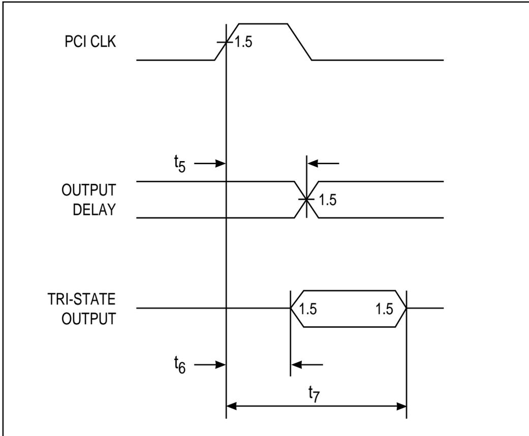
Figure 3. PCI Input Timing
