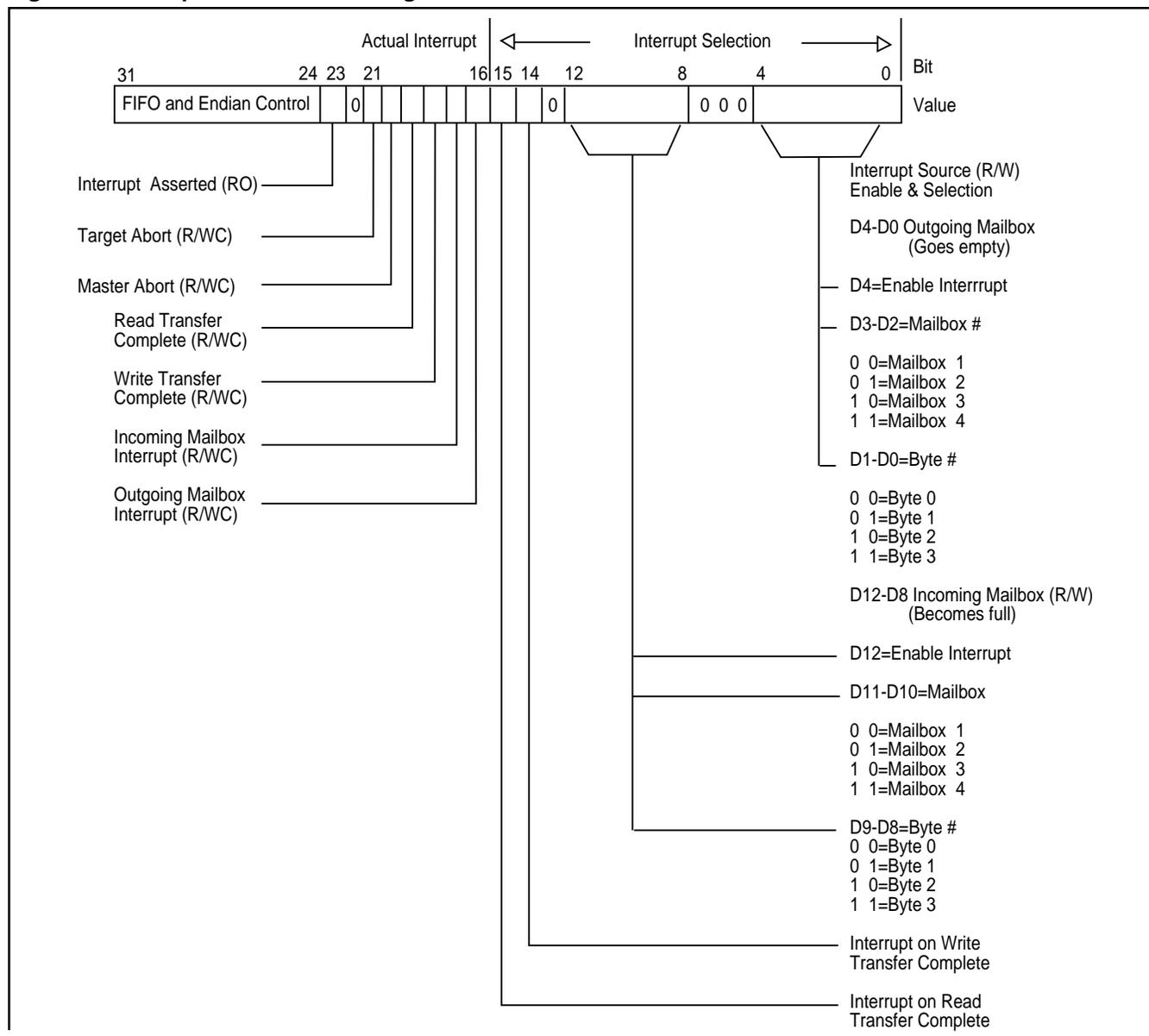
**Figure 7. FIFO Management and Endian Control Byte**
