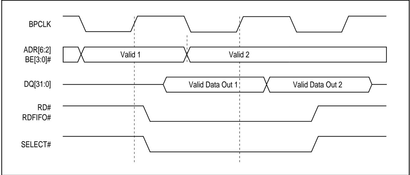
Figure 4. Synchronous FIFO or Pass-Thru Data Register Write
