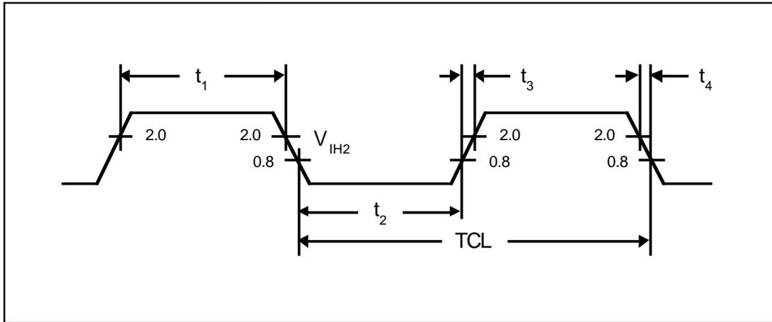
**Figure 5. Pass-Thru Clock Relationship to PCI Clock**
