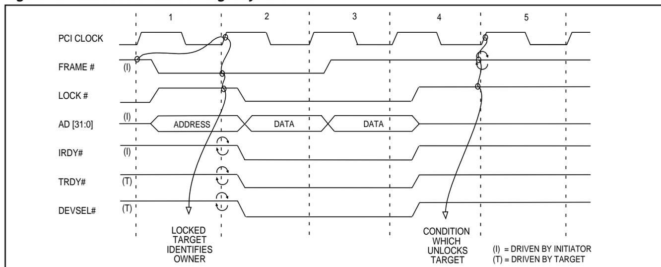
Figure 17. Access Attempt to a Locked Target
