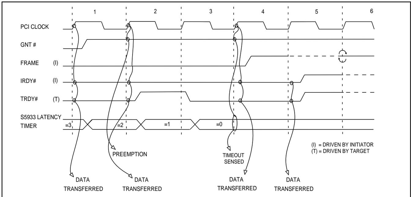
**Figure 8. Master Initiated Termination Due to Preemption and Latency Timer Expired (S5935 as Master)**
