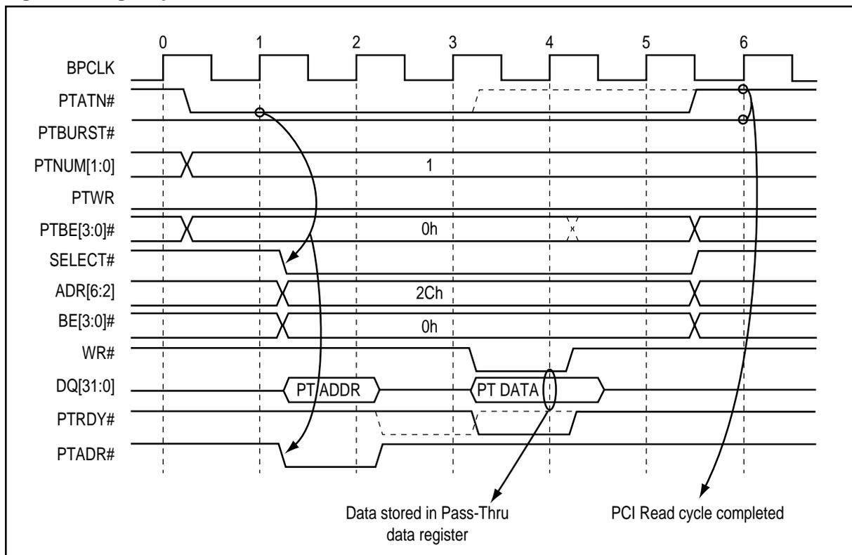
**Clock 4:** If Add-On logic requires more time to write the Pass-Thru data register (slower memory or peripherals), PTRDY# can be delayed, extending the cycle. PTRDY# asserted at the rising edge of clock 4 causes PTATN# to be immediately deasserted and the Pass-Thru access is completed at clock 5.
