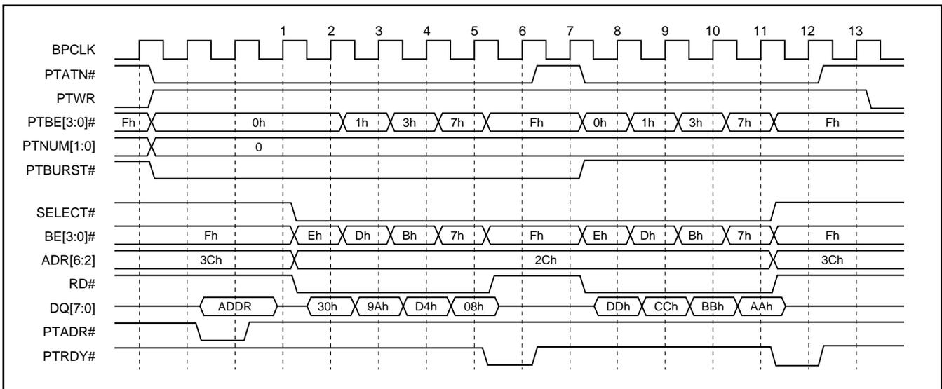
Note: 8 Bit Mode BE's are E, D, B, 7; 16 Bit Mode BE's are C, 3.
