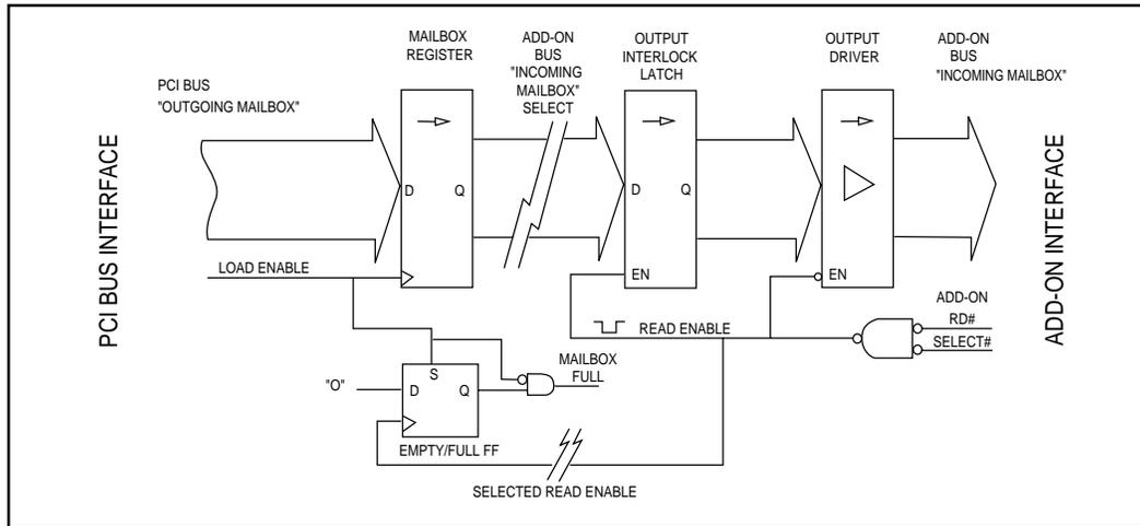
**Figure 2. Block Diagram - Add-On to PCI Mailbox Register**
