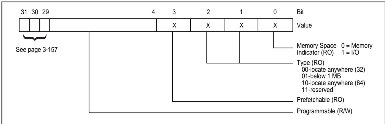
**Figure 11b. Base Address Register — I/O**
