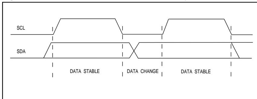
**Figure 3. Serial Interface Byte Access — Write**
