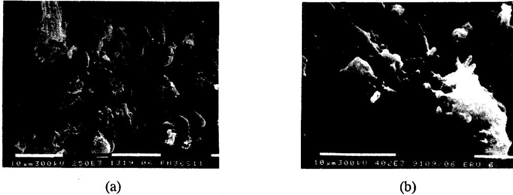
Figure 1: In the first phase of the study, Bacteriae have been observed on corroded calcium carbonate (a). The same morphology has been found in the concrete analyzed during the second phase. In this microphotograph other morphologies can be seen, such as the empty tube at the left side (b).
