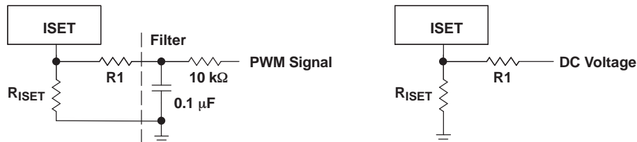
Figure 14. Analog Dimming Uses an External Voltage Source to Control the Output Current
