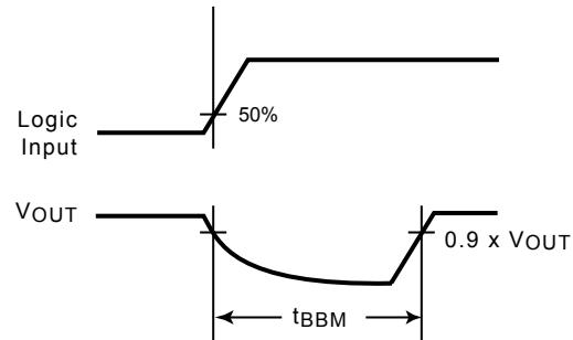
**Figure 3. Break Before Make Interval Timing**
