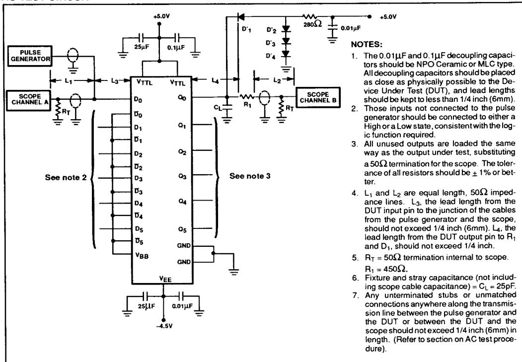
**Translator****100125****ECL INPUT PULSE DEFINITION**
