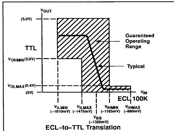
**Translator****100125****AC ELECTRICAL CHARACTERISTICS**Ceramic DIP GND = ground,  $V_{TTL} = 4.5V$  to  $5.5V$ ,  $V_{EE} = -4.8V$  to  $-4.2V$
