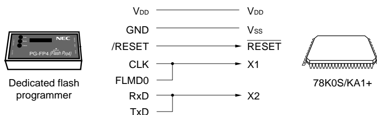
Figure 18-4. Communication with Dedicated Flash Programmer
