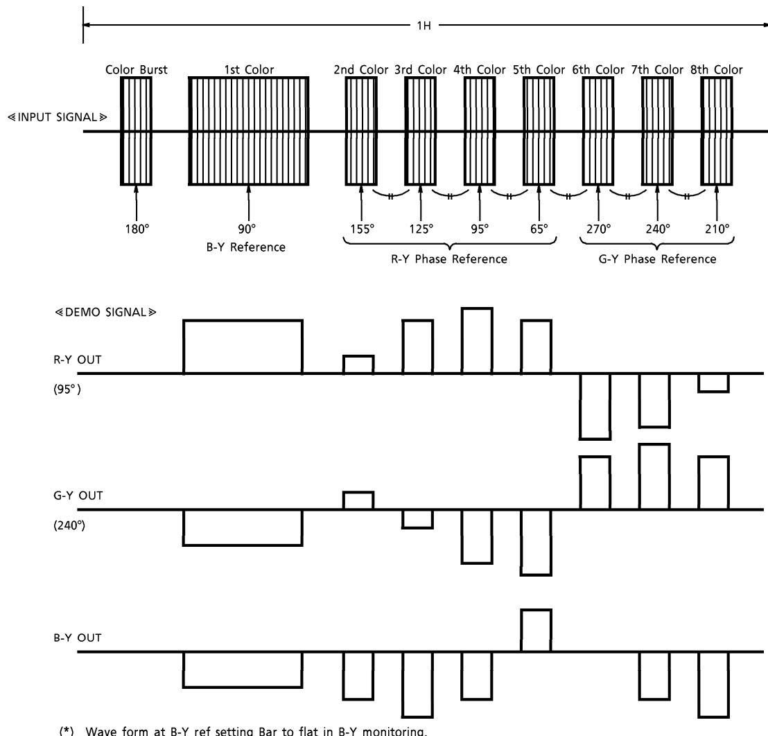
Fig.2 Text measuring signal
