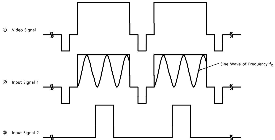
Fig.3 Text test pulse
