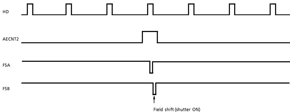
The period of H level on AECNT2 should be longer than the holding period of H level as follows.
