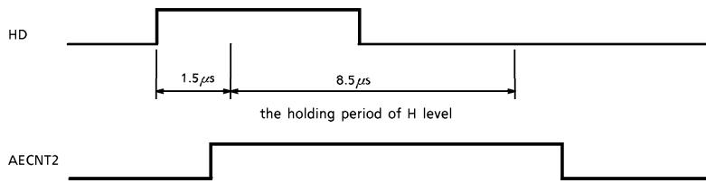
On AECNT mode, generation of trigger pulse needs external counter circuits. And VTG pulse is used for the standard pulse resetting the external counter circuits. The time difference of VTG and field shift (shutter OFF) in the next field are set as follows;
