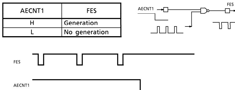
AECNT is not allowed to change while FES pulse is L level. Because AECNT1 gates FES pulse.
