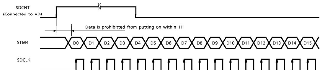
SDCNT is connected to VD of synchronization generator IC.
