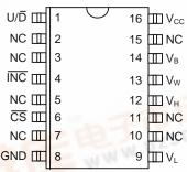
16-PIN SOIC (300 MIL) See Mech. Drawings Section
