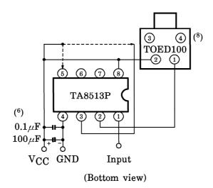
Change the connected pin of TA8513P according to the transmission distance.
