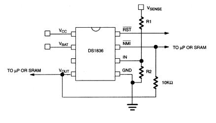
$$V_{\text{SENSE}} = \frac{\text{R1} + \text{R2}}{\text{R2}} \times 1.25$$
