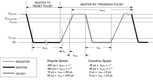
\* In order not to mask interrupt signalling by other devices on the 1-Wire bus, t<sub>RSTL</sub> + t<sub>R</sub> should
