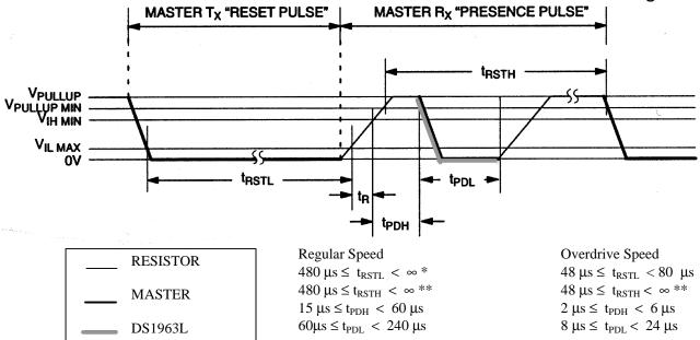
\*IN ORDER NOT TO MASK INTERRUPT SIGNALS BY OTHER DEVICES ON THE 1-WIRE BUS,  $t_{RSTL\,+\,tR}$  SHOULD ALWAYS BE LESS THAN 960  $\mu s$  \*\*INCLUDES RECOVERY TIME
