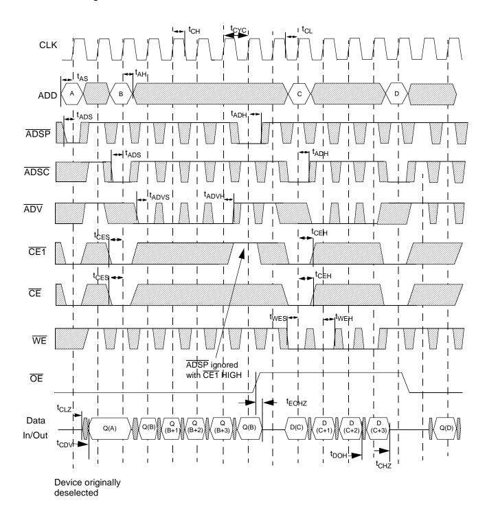
$\overline{\text{WE}}$  is the combination of  $\overline{\text{BWE}}$ ,  $\overline{\text{BWS}}_{[1:0]}$  and  $\overline{\text{GW}}$  to define a write cycle (see Write Cycle Definitions table).  $\overline{\text{CE}}$  is the combination of  $\overline{\text{CE}}_2$  and  $\overline{\text{CE}}_3$ . All chip selects need to be active in order to select the device. RAx stands for Read Address X, WA stands for Write Address X, Dx stands for Data-in X, Qx stands for Data-out X.
