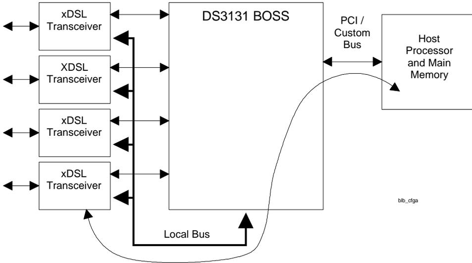
Bridge Mode with Arbitration Enabled Figure 10.1B
