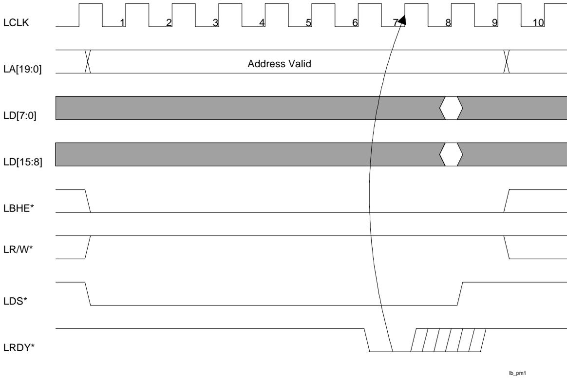
Note: the LRDY\* signal must be detected by the 9th LCLK or the bus access attempted by the Host will be unsuccessful and the LBE status bit will be set.
