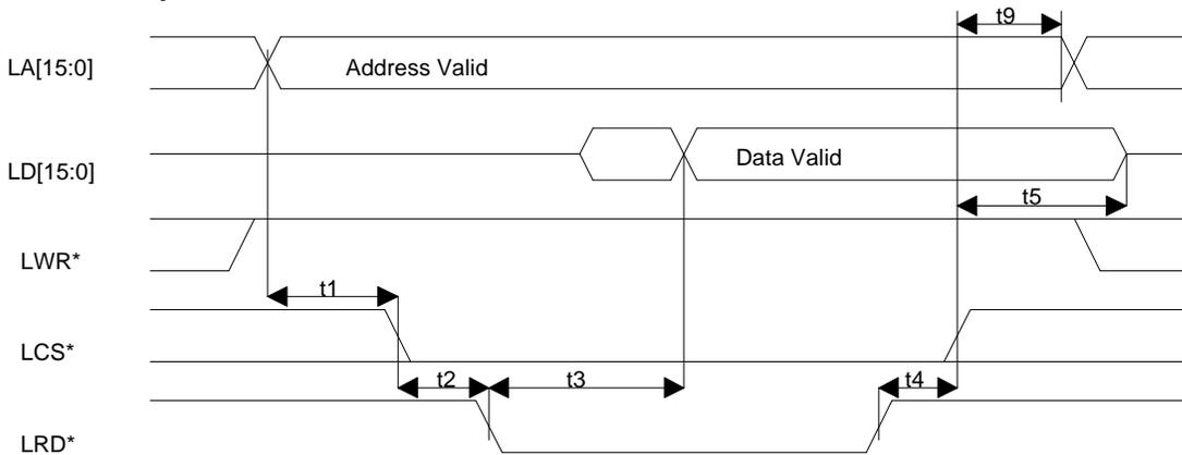
**LOCAL BUS CONFIGURATION MODE (LMS = 1) AC TIMING DIAGRAM** Figure 12C Continued
