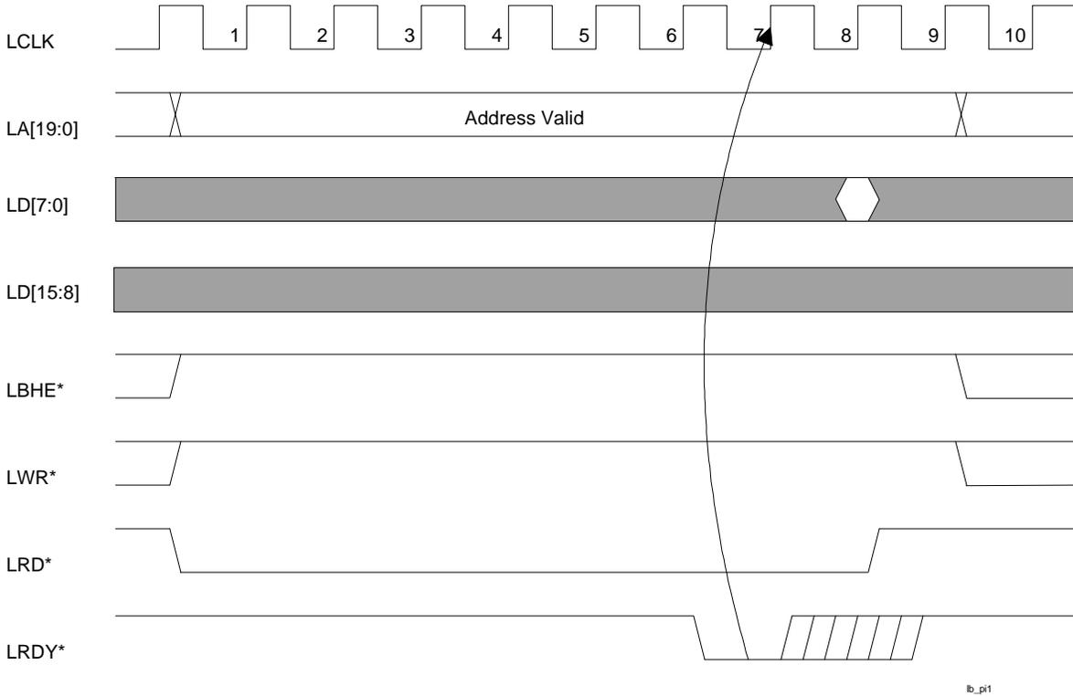
Note: the LRDY\* signal must be detected by the 9th LCLK or the bus access attempted by the Host will be unsuccessful and the LBE status bit will be set.
