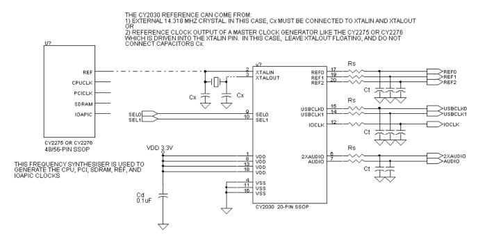
CX = LOAD MATCHING CAPACITORS, REQUIRED WITH EXTERNAL CRYSTALS
