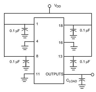
Note: All capacitors should be placed as close to each pin as possible.
