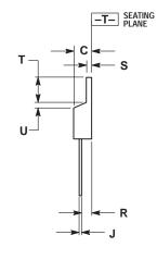
NOTES: 1. DIMENSIONING AND TOLERANCING PER ANSI Y14.5M, 1982. 2. CONTROLLING DIMENSION: INCH. 3. DIMENSION Z DEFINES A ZONE WHERE ALL BODY AND LEAD IRREGULARITIES ARE ALLOWED.
