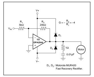
FIGURE 3. Motor Drive Circuit.
