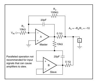
FIGURE 5. Paralleled Operation, Extended SOA.
