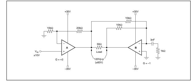
FIGURE 4. Bridge Drive Circuit.
