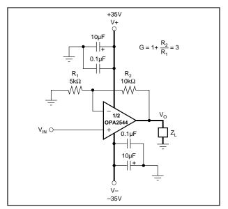
FIGURE 1. Basic Circuit Connections.
