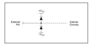
FIGURE 9. Internal ESD Protection.
