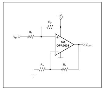
FIGURE 5. DC Level-Shifting Circuit.
