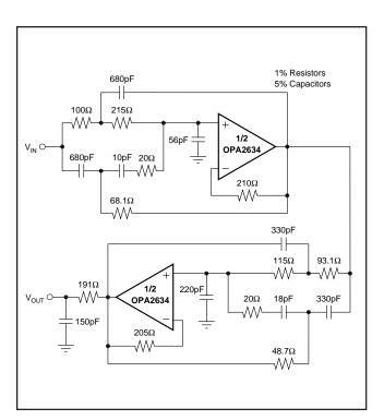
FIGURE 3. Inverse Chebyshev Anti-Aliasing Filter.
