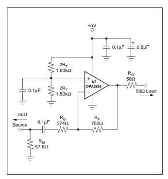
FIGURE 7. Gain of -2 Example Circuit.
