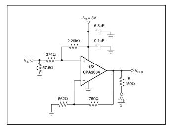
FIGURE 2. DC-Coupled Signal—Resistive Load to Supply Midpoint.
