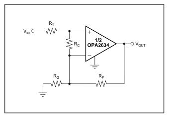
FIGURE 6. Compensated Non-Inverting Amplifier.
