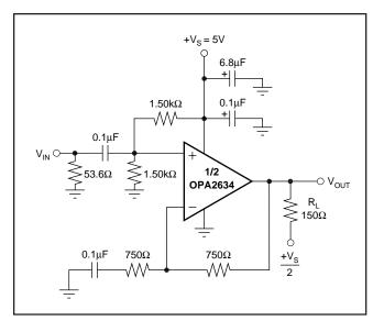
FIGURE 1. AC-Coupled Signal—Resistive Load to Supply Midpoint.
