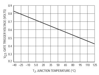
Figure 6. Typical Gate Trigger Voltage versus
