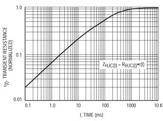
**Figure 4. Transient Thermal Response**
