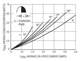
Figure 2. On-State Power Dissipation
