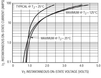
Figure 3. On-State Characteristics
