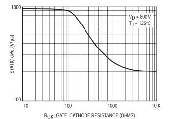
Figure 9. Exponential Static dv/dt versus Gate-Cathode Resistance
