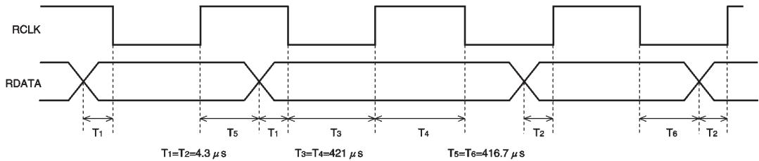
The clock (RCLK) frequency is 1187.5Hz. Depending on the state of the internal PLL clock, the data (RDATA) is replaced in synchronous with either the rising or falling edge of the clock. To read the data, you may choose either the rising or falling edge of the clock as the reference. The data is valid for 416.7μs. after the reference clock edge.
